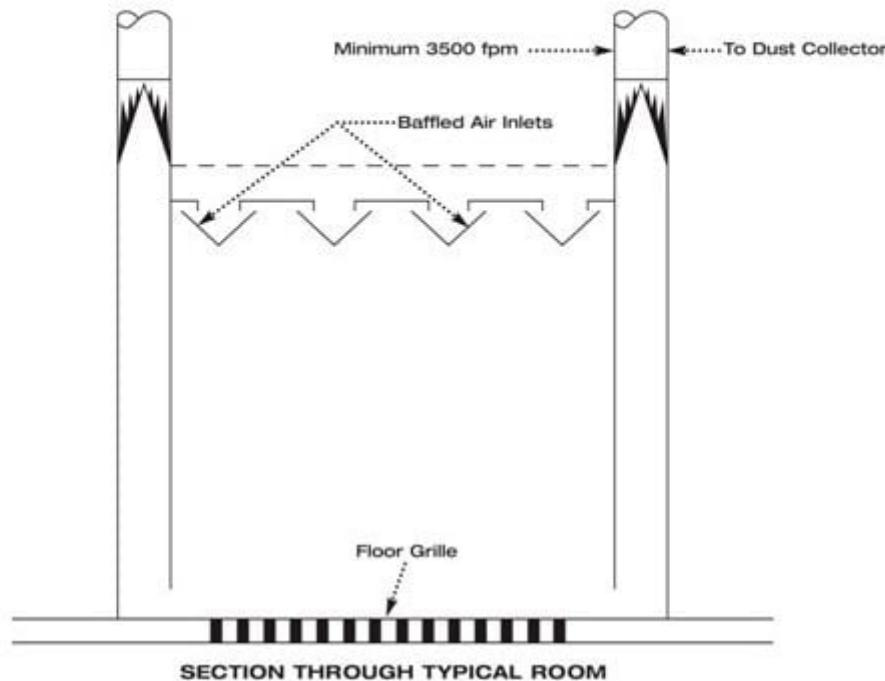
$Q = 50-100 \text{ cfm/ft}^2$  of floor for downdraft with typical choice  $80 \text{ cfm/ft}^2$
