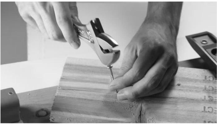
In the image, a person is using an adjustable wrench to drive a screw into a piece of wood while holding the screw in place with bare fingers. This is highly unsafe because the wrench is not designed for this task, and the worker's hand is dangerously close to the point of contact. This method increases the risk of slipping and causing serious hand injuries.
