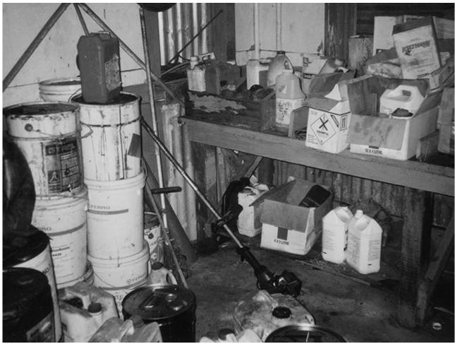
This image shows an unsafe chemical storage area where multiple hazards are present. Containers of different shapes, sizes, and labels are stacked haphazardly, many without proper secondary containment or clear identification. Storing incompatible substances close together increases the risk of dangerous chemical reactions, leaks, or spills—especially in a cluttered, unventilated environment like this.
