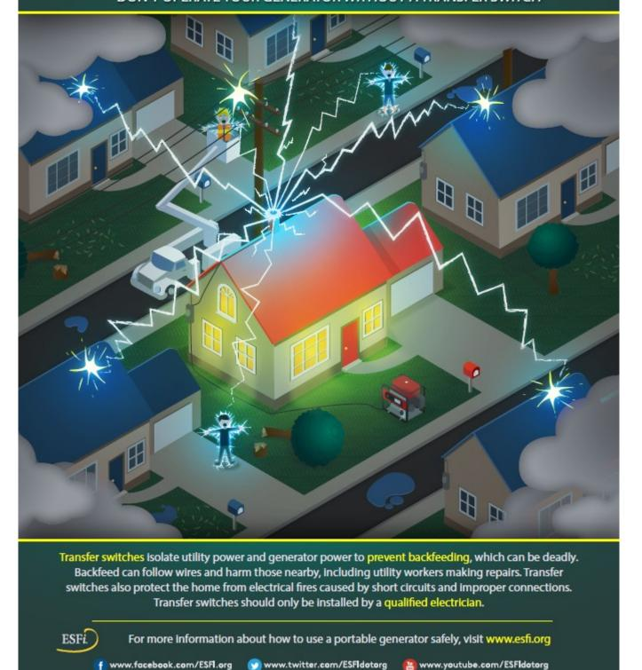
Transfer switches isolate utility power and generator power to prevent backfeeding, which can be deadly. Backfeed can follow wires and harm those nearby, including utility workers making repairs. Transfer switches also protect the home from electrical fires caused by short circuits and improper connections. Transfer switches should only be installed by a qualified electrician.
