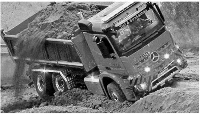
What's wrong in this picture? This truck is about to roll over due to a bad steering wheel maneuver, and the ground where it is operating is too loose for the weight it is carrying.
