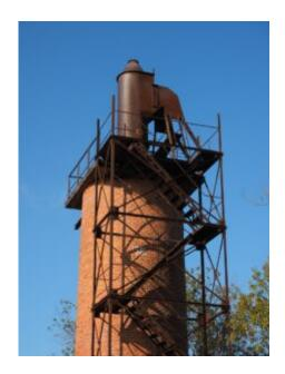
Carbon monoxide killed a supervisor and an engineering draftsman when they entered a lime kiln to check the thickness of the metal walls. The kiln was not blocked off from another nearby kiln which had an induced draft fan in operation. When the two were missed, coworkers put on self-contained breathing equipment and entered the kiln. They found the victims about 160 feet (nearly 50 meters) from the opening.
