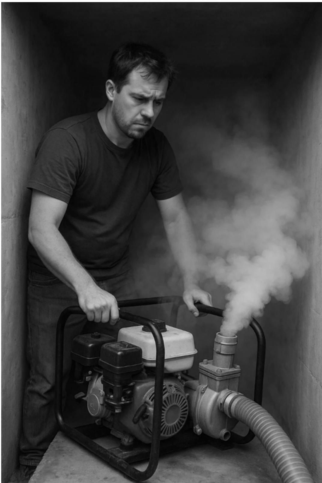
This image shows a person operating a fuel-powered machine in a small, enclosed space with no visible ventilation. The machine emits thick exhaust fumes, which rapidly fill the area. This creates a serious risk of carbon monoxide poisoning, as exhaust gases from internal combustion engines contain toxic fumes that can be deadly when inhaled in confined spaces.
