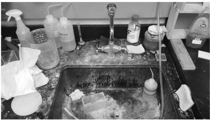
This image shows a major lapse in housekeeping and hygiene in a chemical work area. Contaminated surfaces, unlabelled bottles, and residue buildup around the sink create serious safety risks. Chemicals left unsecured or spilled can lead to cross-contamination, reactions, skin burns, inhalation hazards, and even accidental poisoning. Poor hygiene in such areas also increases the likelihood of environmental contamination and regulatory violations.
