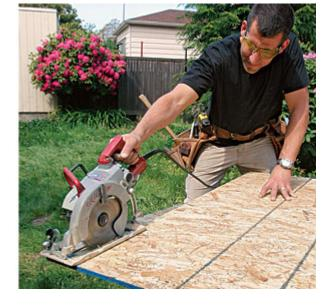
**Prevention strategy:** Keep the blade sharp, use the saw at the speed the manufacturer recommends and properly support the stock being cut—remember, using your legs is not a proper means of support!
