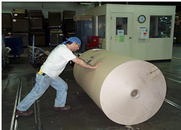
These paper rolls weigh about 3,000 pounds. Just imagine how much stress it puts on the worker's back, shoulders, arms and wrists to roll these monsters by hand—especially across a concrete, sloped floor that's pocked with holes and latticed with roll stand tracks! It's a musculoskeletal disorder (MSD) just waiting to happen.
