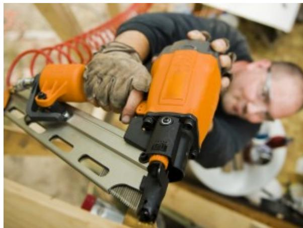
**3. Single Sequence Triggers** which like full sequential triggers, will only fire when the controls are activated in a certain order. First, the safety contact tip must be pushed into the work piece. Then, you must squeeze the trigger. To fire a second nail, you only need to release the trigger.
