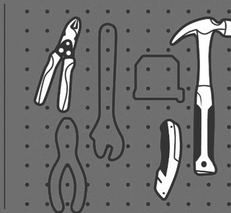
Examples: A peg board with visual outlines of hand tools in bright colors. Each workstation should be designed for an economy of motion. Make a diagram of lines showing distance from tool crib, materials and finished goods across the entire shop floor.
