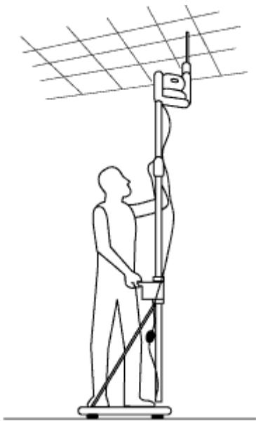
Tool support eliminates over-stretching and overreaching.
