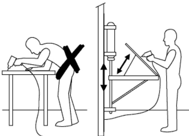
Workbench with adjustable height and tilt improves working position.
