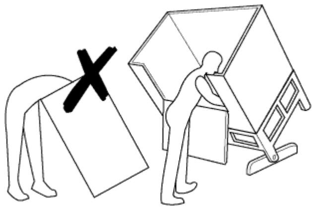
Lift-and-tilt device and side opening on bin reduces bending.
