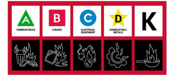
Class A fire extinguishers are used for ordinary combustibles such as wood, paper, some plastics and textiles. This fire class requires the heat-absorbing effects of water or the coating effects of certain dry chemicals. According to NFPA, extinguishers suitable for Class A fires should be identified by a triangle containing the letter "A." If in color, the triangle should be green.
