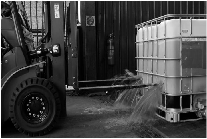
This image highlights the critical importance of conducting pre-operation checks on powered industrial trucks like forklifts. Here, the forklift's forks have punctured a container, causing a significant hazardous material spill. This incident could lead to environmental contamination, worker injury, or even fire if the substance is flammable.
