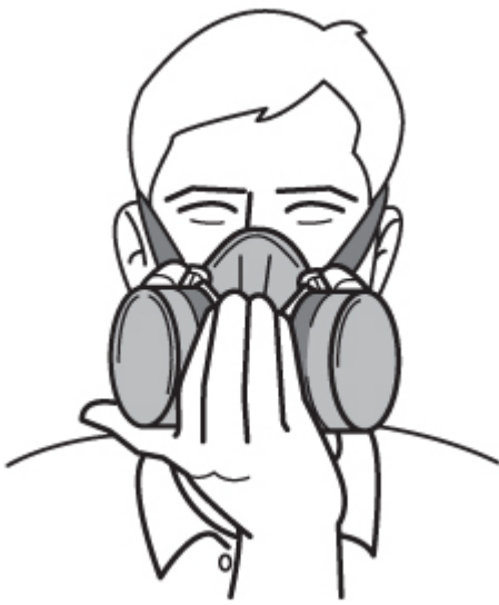
Figure 4: Positive pressure fit check
