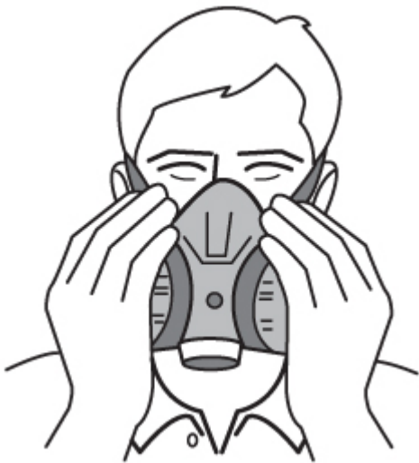
Figure 3: Negative pressure fit check
