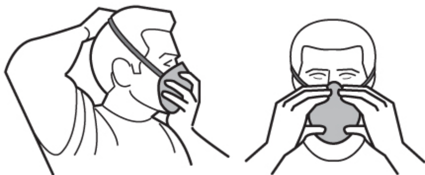
Figure 2: How to put on a disposable respirator
