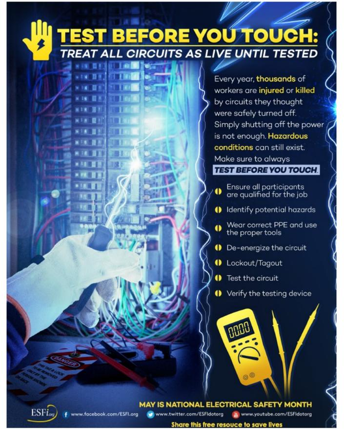
Every year, thousands of workers are injured or killed by circuits they thought were safely turned off. Simply shutting off the power is not enough. Hazardous conditions can still exist. Make sure to always **TEST BEFORE YOU TOUCH.**
