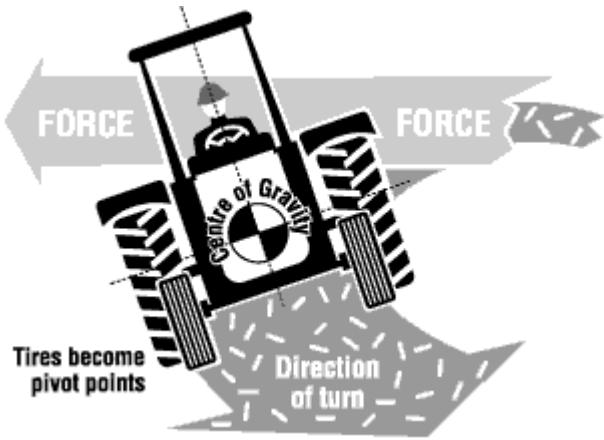
The outward tipping force varies according to the tractor speed and turning radius. Sharp turns increase the force.
