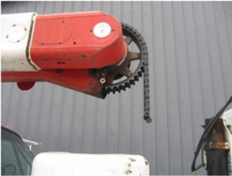
Photo 2: Broken boom actuating chain (photo courtesy of OSHA).
