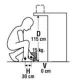
To calculate the recommended weight limit (RWL) for the task:
